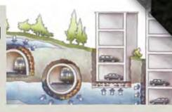
For relief of hydrostatic pressure in vertical foundation applications
